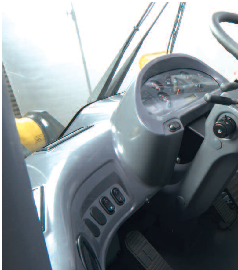
1: Cut-off ON/OFF switch 2: Cut-off adjustment switch 3: Fan reverse ON/OFF switch 4: Boom control 5: Bucket control
